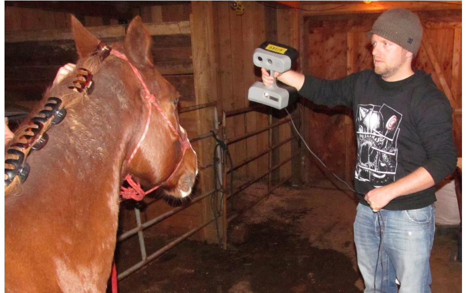
Alex Shvartzman uses a handheld structured light device to scan a horse Image from: https://cinefex.com/blog/lidar/
