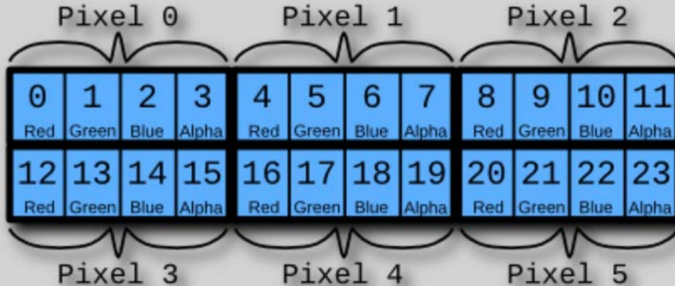
Pixel layout in the pixel array for a 3-by-2 image of 6 pixels. Each pixel takes 4 elements in the array for red, green, blue, and alpha, for a total of 24 array elements, 0-23.
